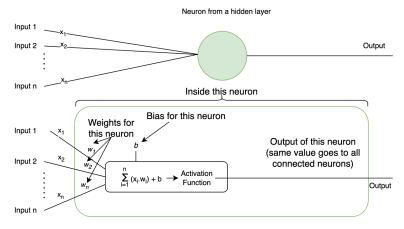
Figure 6.9 Feed-Forward Cell.
