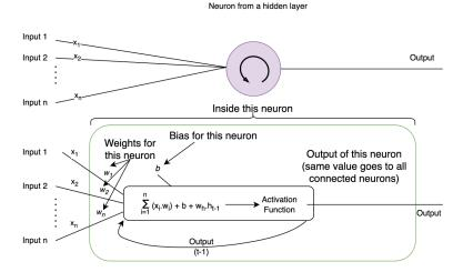
Figure 6.10 Recurrent Cell.
